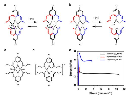
**Fig. 3** Control experiments for mechanism study. **a**, **b** Two energy dissipation process for [Zn(Hbimcp)<sub>2</sub>]<sup>2+</sup>. **c** The molecular structure of [Zn<sub>2</sub>(bimcp)<sub>2</sub>Cl<sub>2</sub>]. **d** The molecular structure of [Ni(Hbimcp)<sub>2</sub>]<sup>2+</sup>. **e** Comparison of stress-strain curves for **Zn(Hbimcp)<sub>2</sub>-PDMS**, **Ni(Hbimcp)<sub>2</sub>-PDMS** polymer, and **Zn<sub>2</sub>(bimcp)<sub>2</sub>-PDMS**
