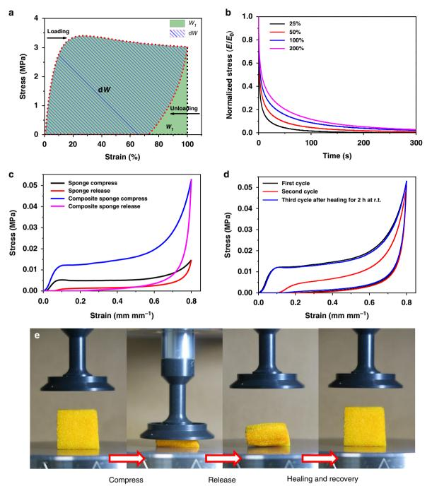
**Fig. 4** The energy absorbing properties of Zn(Hbimcp)<sub>2</sub>-PDMS polymer. **a** The calculation of energy absorbing efficiency. **b** Normalized stress-relaxation curves under different strain. **c** Cyclic strain-stress curves of blank sponge and composite sponge. **d** Cyclic strain-stress curves of composite sponge with healing process. **e** Optical images of the composite sponge under compression, healing, and recovery processes
