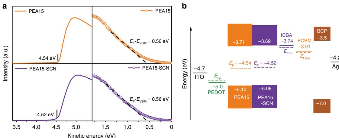
**Fig. 2 Band structure of tin PSCs.** **a** UPS spectra of secondary electron cutoff and valence band of perovskite films. **b** Schematic illustration of energy levels. Dashed lines represent the quasi-Fermi level of ICBA ( $E_{Fn-i}$ ), PCBM ( $E_{Fn-p}$ ), and PEDOT ( $E_{FP}$ ).
