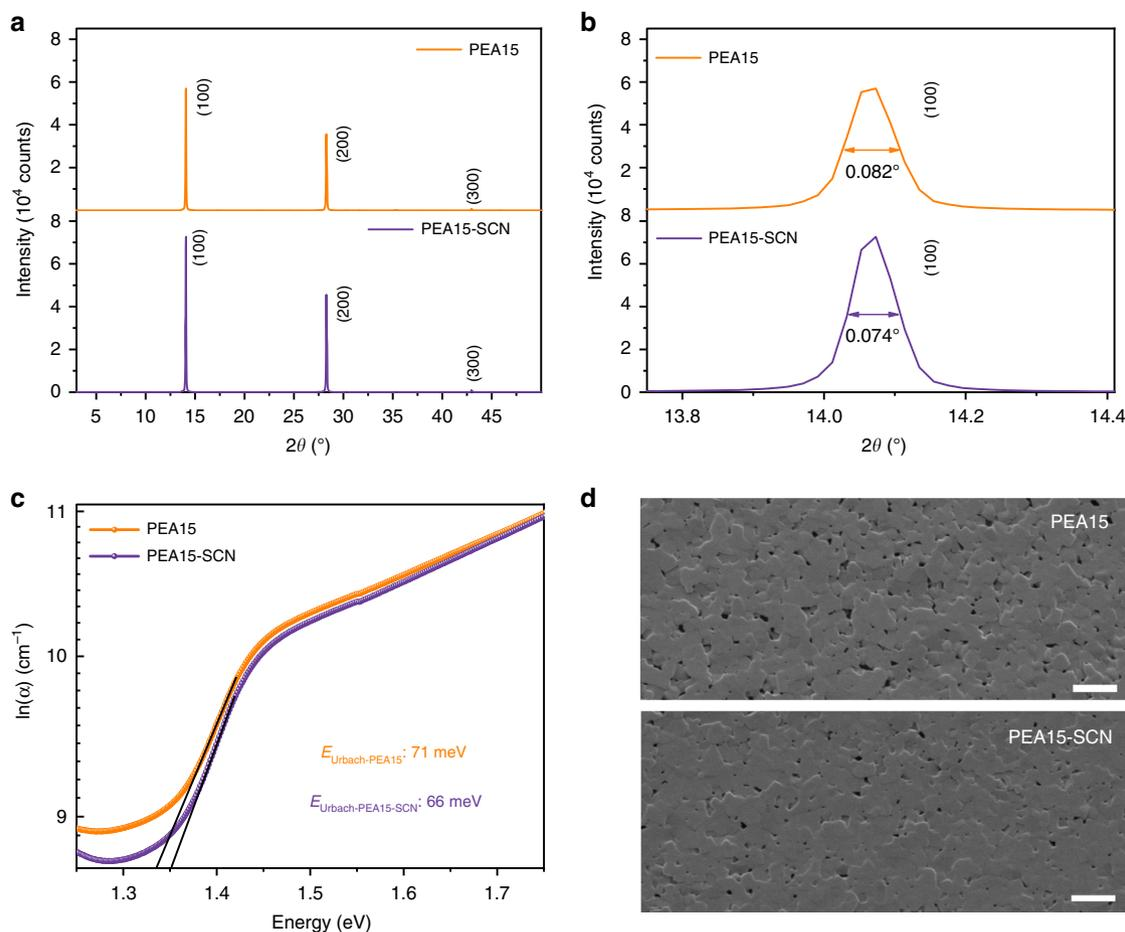
**Fig. 1 Perovskite film characterization.** **a** XRD spectra of perovskite films and **b** the corresponding FWHM values of (100) peak. **c** The Urbach energy of perovskite films. **d** SEM images of perovskite films. The scale bar is 1 μm.
