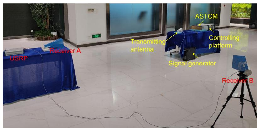
**Fig. 9 | Experimental scenario of data transmissions at two frequencies toward different deflection angles.** The ASTCM is illuminated by a transmitting horn antenna at 4.25 GHz, which is connected to a signal generator. The ASTCM is
