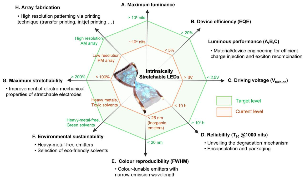
**Fig. 2 | Future directions for intrinsically stretchable LEDs.** a Challenges for intrinsically stretchable LEDs. b Technical pathways for intrinsically stretchable LEDs.  $V_{\text{turn-on}}$ , device turn-on voltage;  $T_{90}$ , device lifetime for the brightness to decrease to 90% of its initial value. FWHM, full-width half-maximum.
