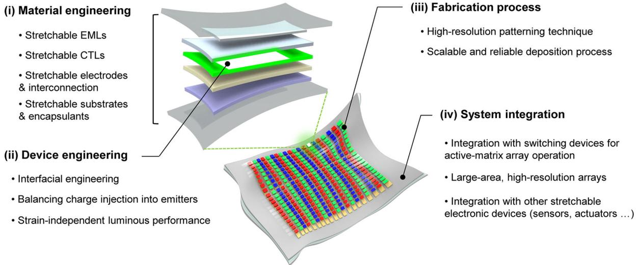
**b. Technical pathways for intrinsically stretchable LEDs**
