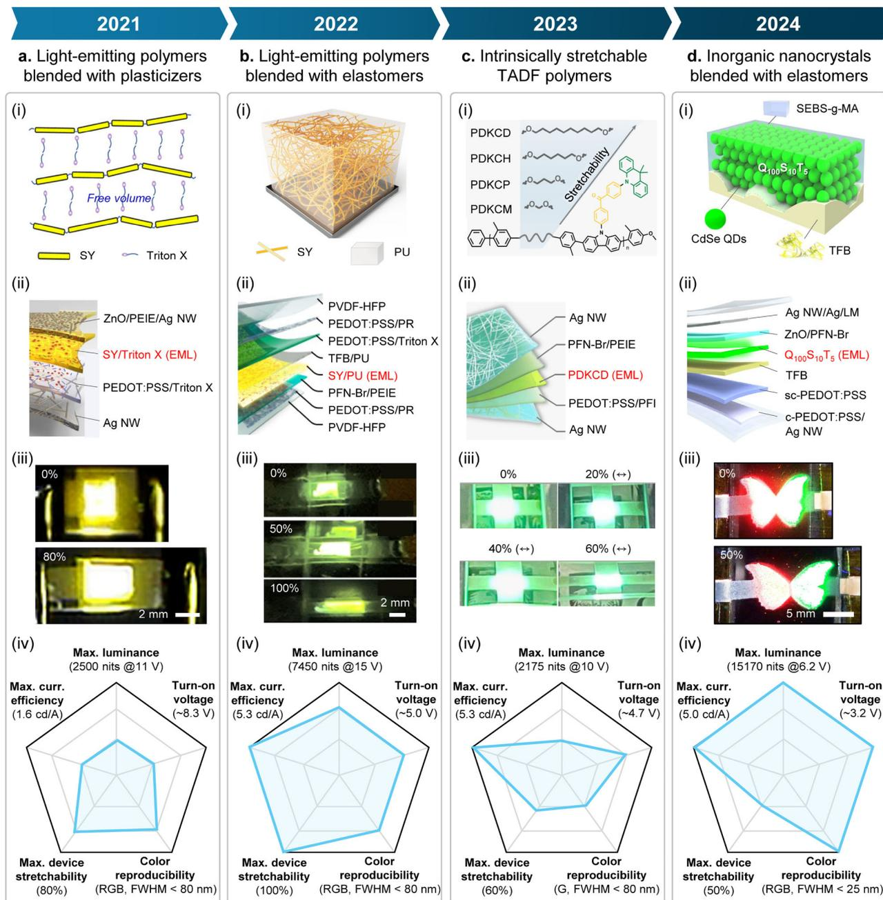
**Fig. 1 | Recent advancement on intrinsically stretchable EL materials and their device applications.** **a–d** Key approaches for intrinsically stretchable LEDs. For each approach, material strategies for stretchable EMLs (i), device structures of intrinsically stretchable LEDs (ii), photographs of device operation under the applied strain (iii), and comparative evaluation of device performance (iv) are provided.
