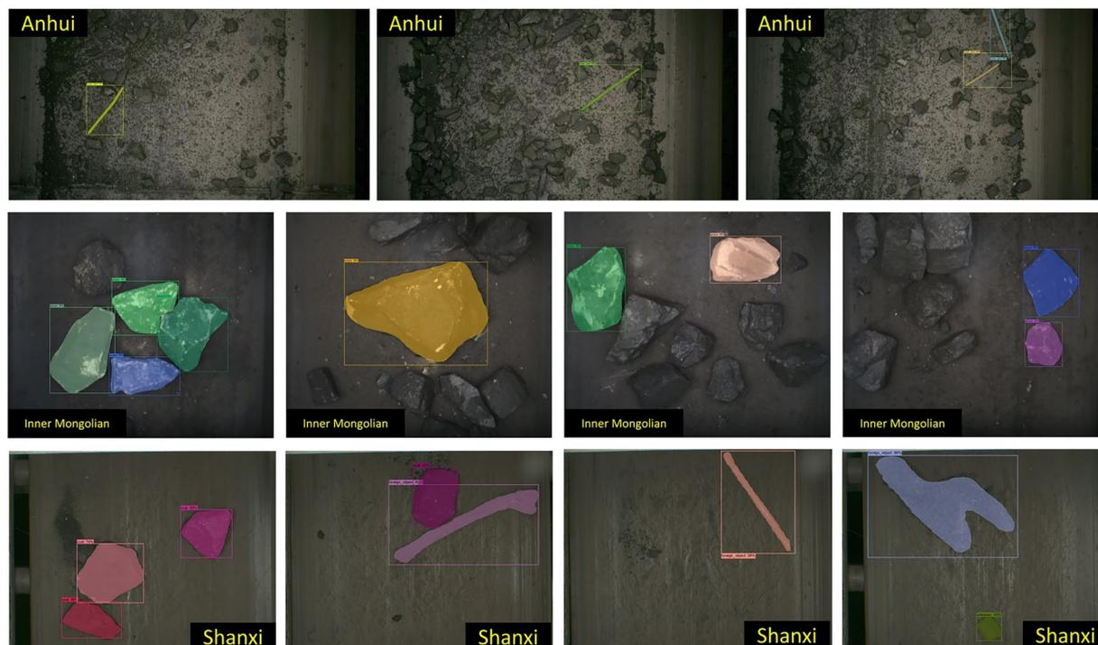
**Fig. 7** The samples of test results of instance segmentation.
