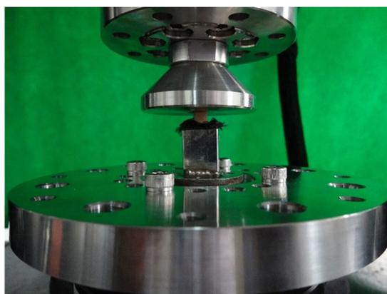
**Figure 9.** Biomechanical test of the bone block.
