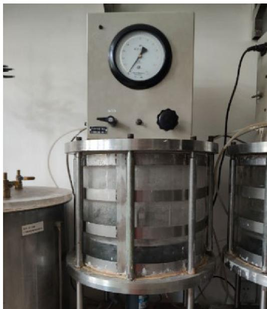
**Figure 2.** YRK-1 rock dissolution apparatus.
