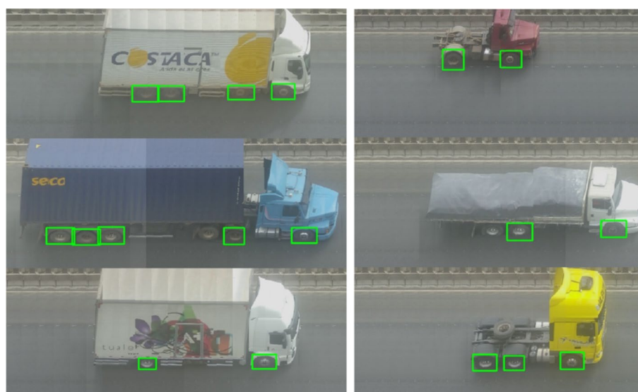
Figure 8. Axle counter inference in real images.
