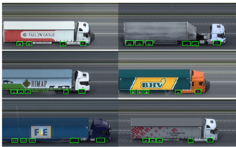
Figure 7. Axle counter inference.
