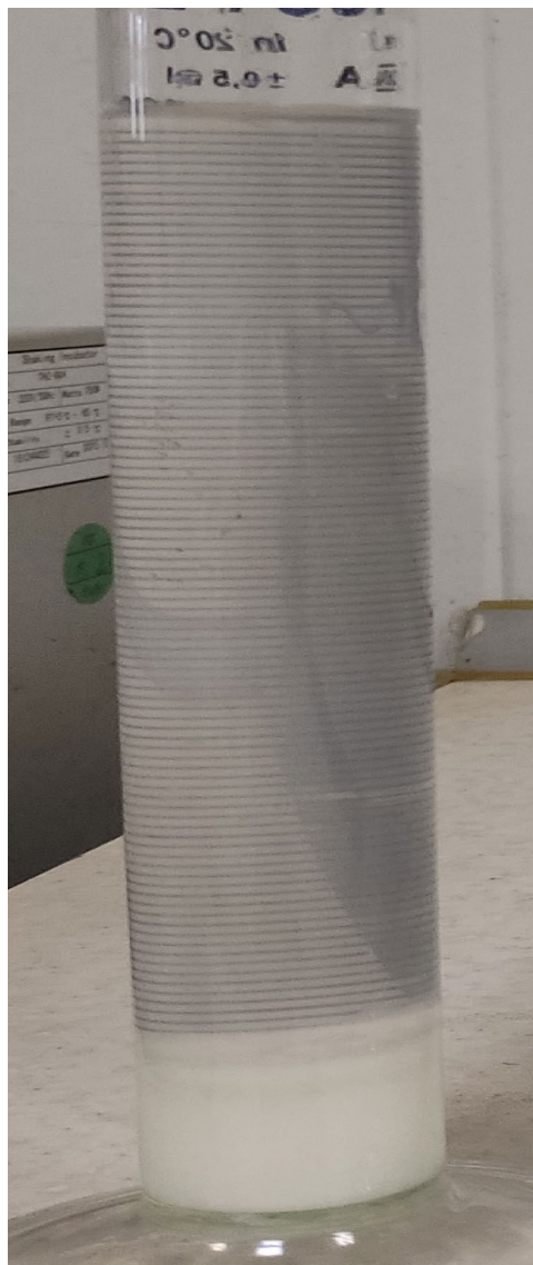
Fig. 2. Settlement of 250 ppm MgO nanoparticles fluid after 10 min.
