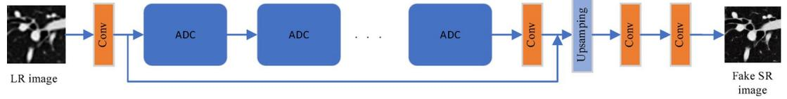
**Fig. 1.** Structure of the generator network.
