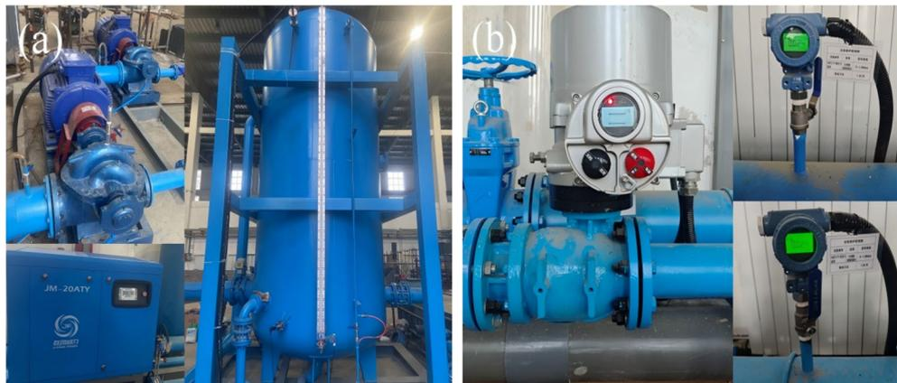
**Fig. 5.** Water hammer test platform equipment: (a) Multi-functional Variable-head System; (b) terminal valve with upstream/downstream pressure transducers.
