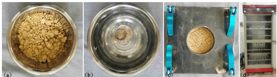
**Fig. 12.** Indoor direct shear test. (a) Fully stir the sample; (b) The sample was stuffed in water for 24 h; (c) Rough treatment of the layered interface; (d) Constant temperature and humidity curing for 7 days.
