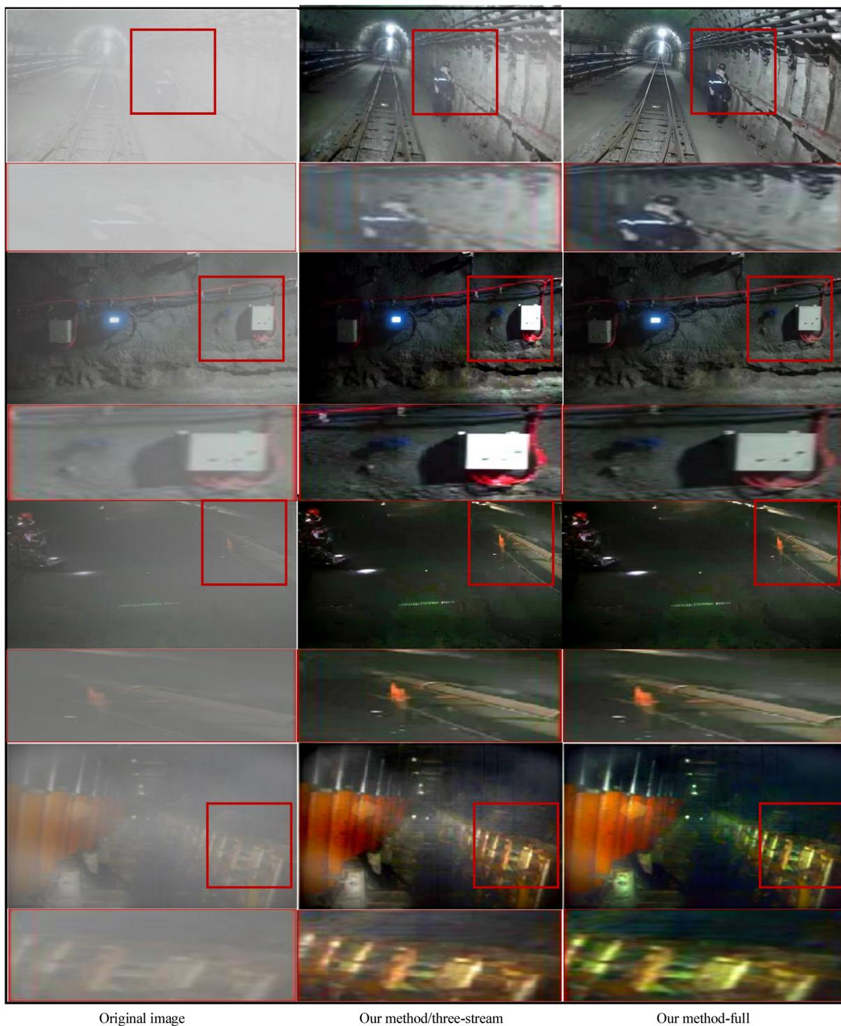
**Fig. 9.** Dehazing results of our method and the remove three-stream branching method on coal mine dust images.
