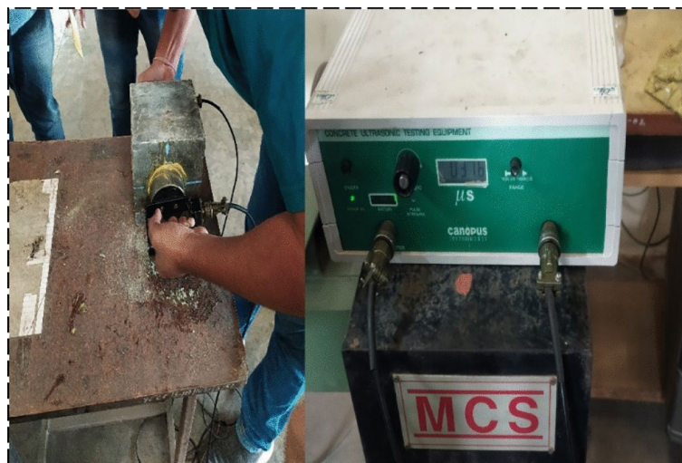
Fig. 21. UPV testing on concrete cubes.
