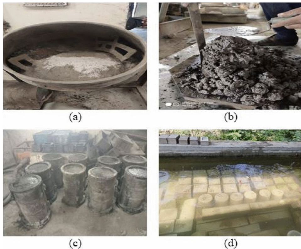
Fig. 6. Casting of Specimens (a) Dry Mixing, (b) Slump Determination, (c) Casting, and (d) Curing.
