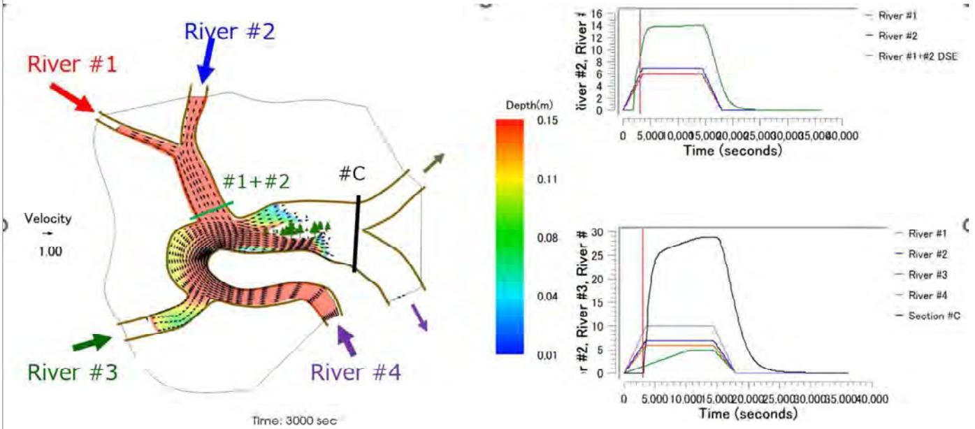
It is possible to display the discharge at any cross-section.
